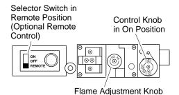
Figure 49 - Setting the Selector Switch, control Knob, and Flame Adjustment Knob for Remote Operation
